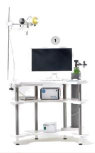
Safe auto zeroing means, the patient can breath during the zeroing procedure. Ambient conditions sensors make the input of these data unnecessary. We want to make the lung function testing as safe and simple as possible.
